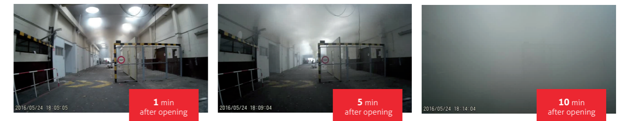
Test No. 3 Change in visibility during a test involving cool smoke ( 2\% \Sigma A_a )
