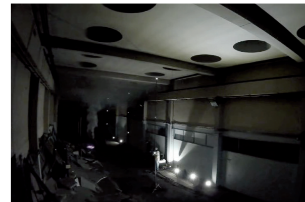
Test No. 8: distributed roof vents Heat output: 150 kW 0.5% \Sigma A_a
